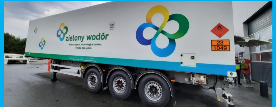
Hydrogen trailer with the capacity of 1000 kg
