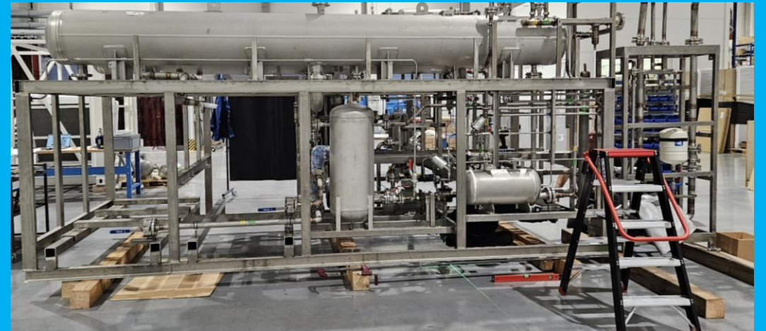
Hydrogen bus factory | 0.5 MW alkaline electrolyzer
