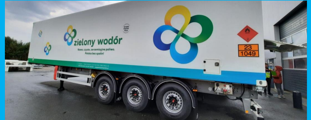
Hydrogen trailer with the capacity of 1000 kg
